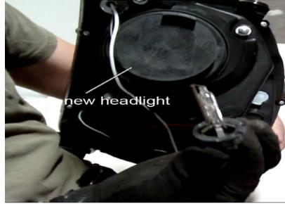
Install the Xenon Harness to the new Housing, run the wire to the bottom of the housing where the ballast is located.
