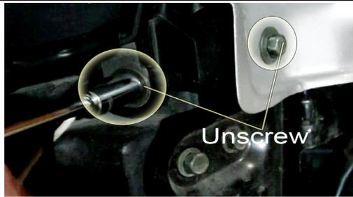
Unscrew the bottom inner headlight assembly
