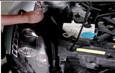
On the Bottom of the Headlight, the other end of the Ground wire should be connected to the screw that holds the headlight housing.
