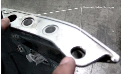
On the bottom of the bumper, there are 10 screws to remove. Using a philip screwdriver or a 10mm socket.
