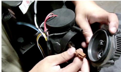
Plug the Ballast socket back on, and before screwing the ballast, connect the **GROUND WIRE** to the ballast. Be sure to connect it on the outer part of the head light.(as shown) The other end of the Ground will be connected to the housing.
