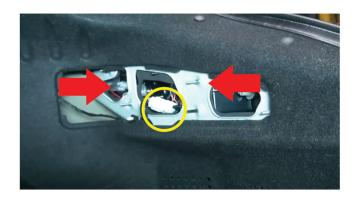
6) Carefully mount the new Spyder LED tail light back onto the body of your car. Make sure to line up the holes and replace the 4 10mm screws. Reconnect the new harness to the OEM harness as well. Lastly, replace the tail light panel cover, test for connectivity, and you're done. You have now successfully installed your new LED tailights to your Hyundai Genesis coupe.
